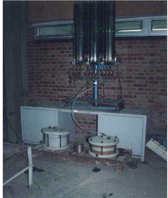
Fig. 2. Permeability test in large-scale model.
