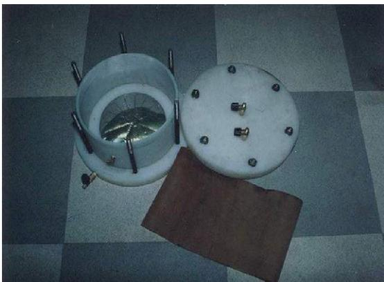
Fig. 1. Model container and rubber membrane.
