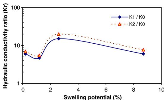
Fig. 8. Hydraulic conductivity ratio versus swelling potential of test soils.
