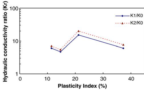
Fig. 5. Effect of soil plasticity indices on post desiccation hydraulic conductivity ratio.
