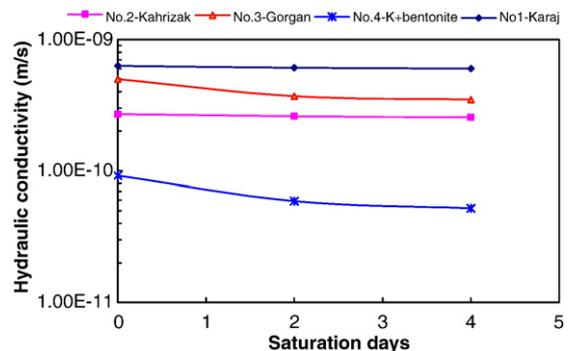
Fig. 7. Hydraulic conductivity of desiccated test soils following 2 and 4 days of saturation.
