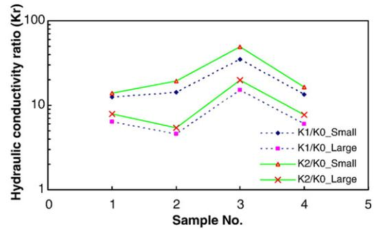
Fig. 9. Hydraulic conductivity ratio of specimens with different sizes.
