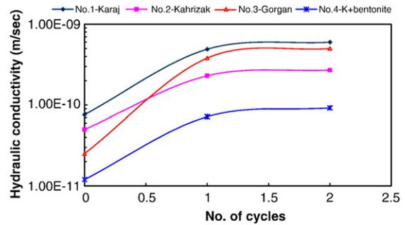
Fig. 4. The hydraulic conductivity records for different cycles of drying and wetting.
