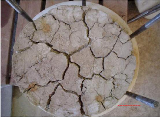
Fig. 3. Crack distribution in soil model No. 3 (Gorgan).
